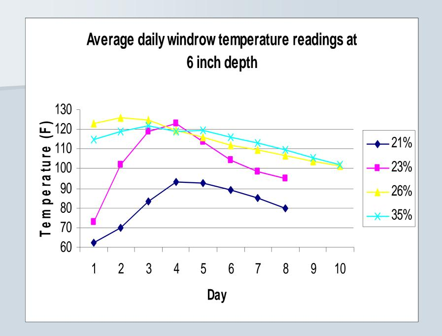
Average daily windrow temperatures during 10 days of inhouse pasteurization of poultry litter at various moisture levels
