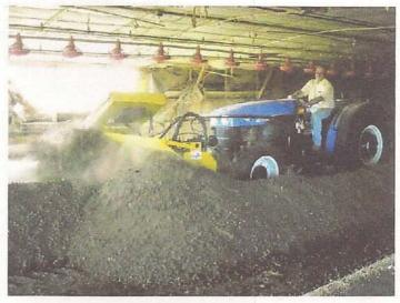
Figure 1. In-house composting of litter using Brown Bear aeration equipment.
